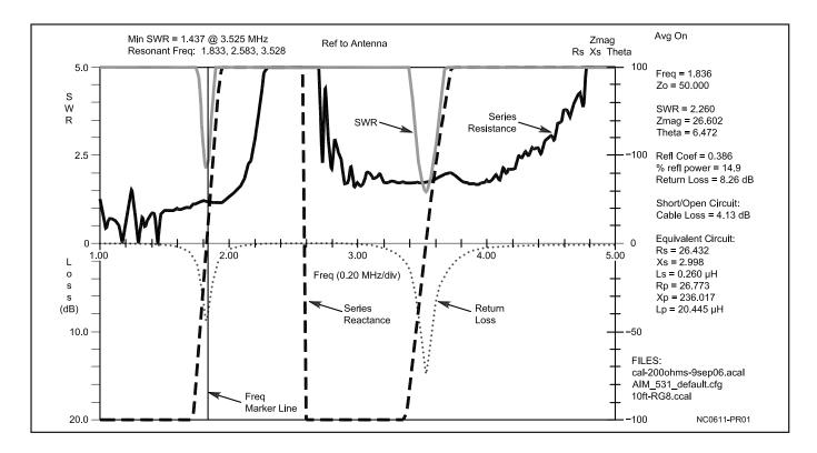
SWR, return loss, series resistance and series reactance. The data on the right side of the plot is for the frequency of the vertical marker line.
